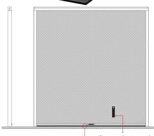
When the bottom pull rod is locked in the lowest position, there should be no gap between it and the base surface.
