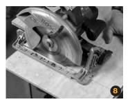
**Cut panels to accommodate shower heads and faucets.** Measure and mark the borders where the opening will be with a marker. Drill a 1/2-inch to 1-inch hole using a drill in a corner of the cut-out section (image 9). Use a jigsaw or hole saw to cut the remaining opening, following your tracing (image 10, 11).
